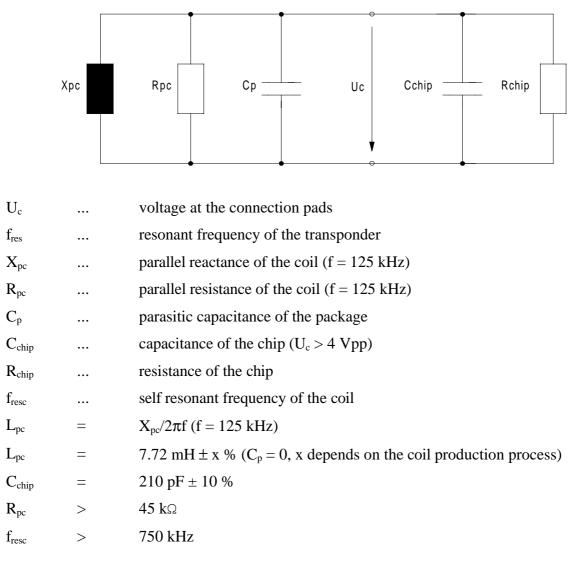
Note: The parasitic capacitance of the package (C<sub>p</sub>) must be considered.
